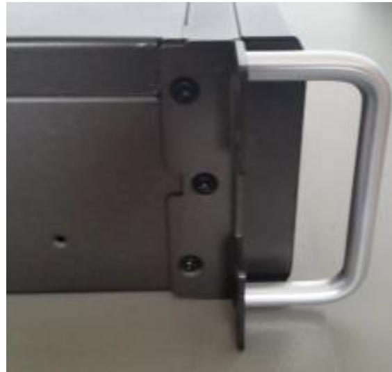
FIGURE 4 Attach the mounting bracket and handle
